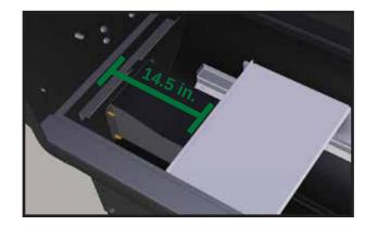
Improper shield placement will result in issues coming to temperature. When using the heat shield adjustment rod, a centered heat shield should be positioned approximately at the "0" mark on the rod, setting the heat shield roughly 14.5 in. (368.3 mm) from the left inside grill wall. The depth to which the rod is threaded into the receiving nut varies, so some experimenting might be needed to find the perfectly adjusted center point on your rod.
