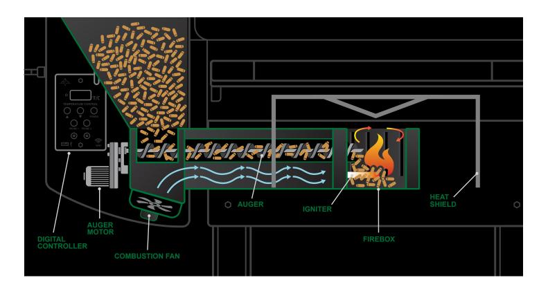
The beauty starts at the core of GMG's 12V Direct Power design. Direct current allows for a micro-adjusted variable speen fan and auger motor that creates more precise temp control, greater fuel economy, and less waste along with increased motor RPM's for quicker pellet feed and faster startups.
