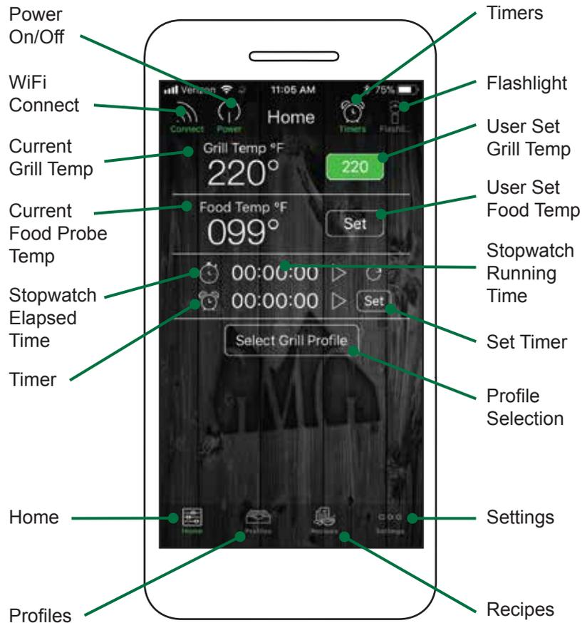
The control screen allows you to turn your grill on/off, set the grill temperature, set the food probe temperature, and set a timer or stopwatch.
