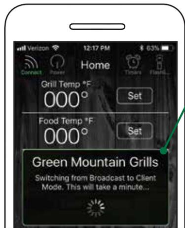
Now that the grill is in broadcast mode, the next step is to switch it to the client mode. This step requires the grill to briefly disconnect and reconnect to the router with a new configuration, which takes around a minute.
